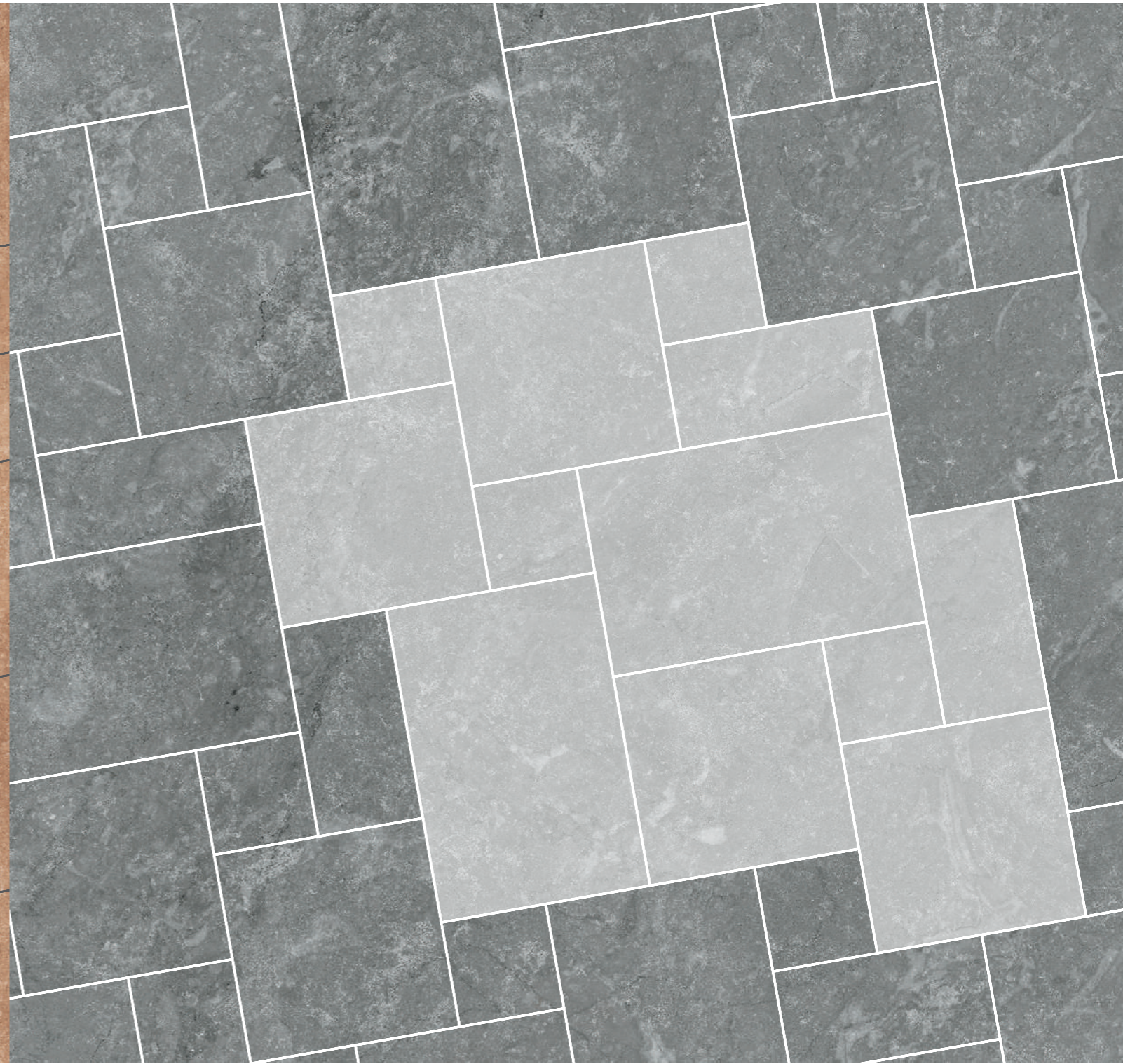
MODULO 4 11% MQ 20x20 8"x8" | 11% MQ 20x40 8"x16" | 44,50% MQ 40x40 16"x16" | 33,50% MQ 40x60 16"x24" si consiglia posa con fuga 3/4 mm | suggested laying with 3/4 mm joint | pose conseillée avec 3/4 mm de joint
